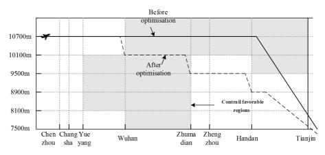
Fig. 7. The flight profile comparison before and after optimization
