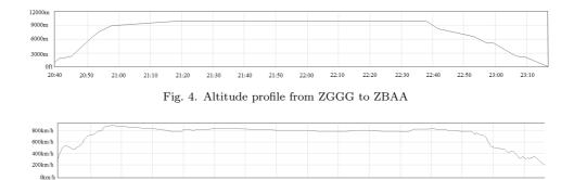
21:50 Fig. 5. Velocity profile from ZGGG to ZBAA
